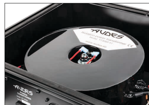
The 3kVA toroidal transformer is a caliber you don't see every day
