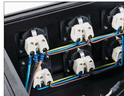
The sockets are wired together with thick solid conductors
