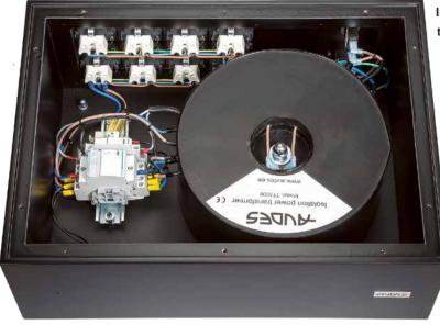
Inside, we discover a balanced toroidal transformer with impressive dimensions that contribute the lion's share to the 33 kilograms the device weighs in at.
